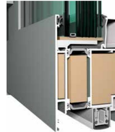
The CS 77-FP EI30 and EI60 is developed based on the existing CS 77 profiles and accessories for windows and doors and extensively tested in an optimized European test and approval program. The fireproofing time span is achieved by inducing a special cooling material into the profile chambers and by using self-adhesive and water-resistant swelling gaskets. These gaskets do not need to be sealed, reducing fabrication time of the profiles and saving costs.
