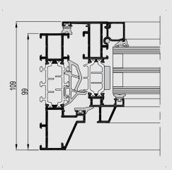
SlimLine 38 is a highly insulated system inward and outward opening windows and doors, which combines elegance and comfort, with a unique design. This special slender steel look is the perfect solution for modern architecture and renovation of steel-framed windows, respecting the original design but offering a thermally improved solution.
