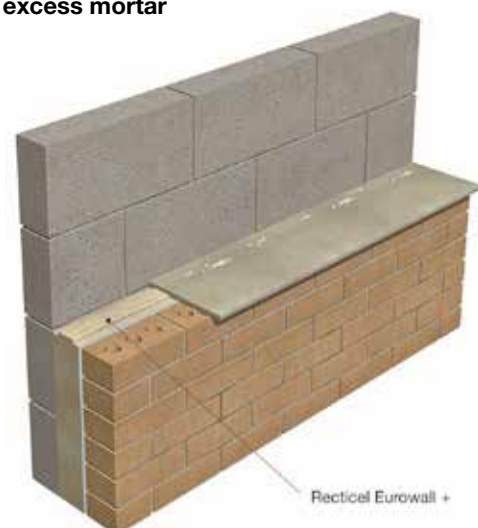
Fig. 3. Use of a cavity board when cleaning off excess mortar
