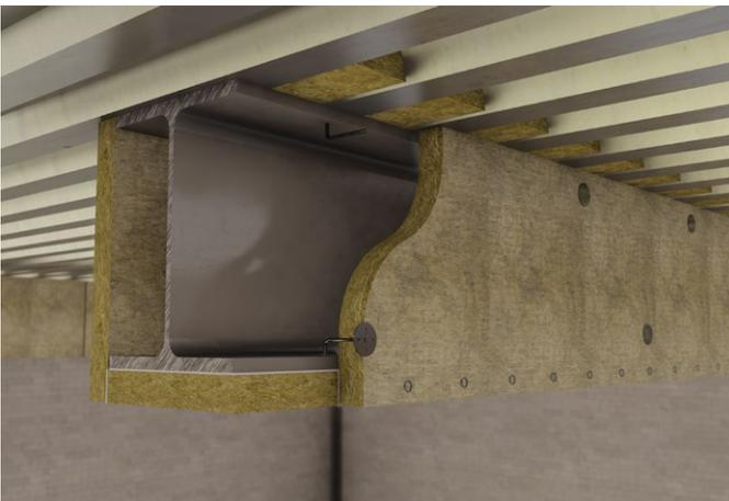
**Figure 6 -** Stud welded pin dry joint board system (Up to 2 hours fire protection)
