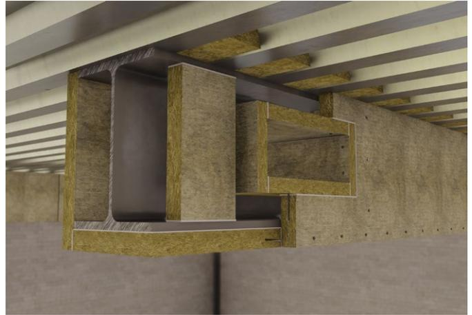
**Figure 12** - Beam with square or rectangular holes
