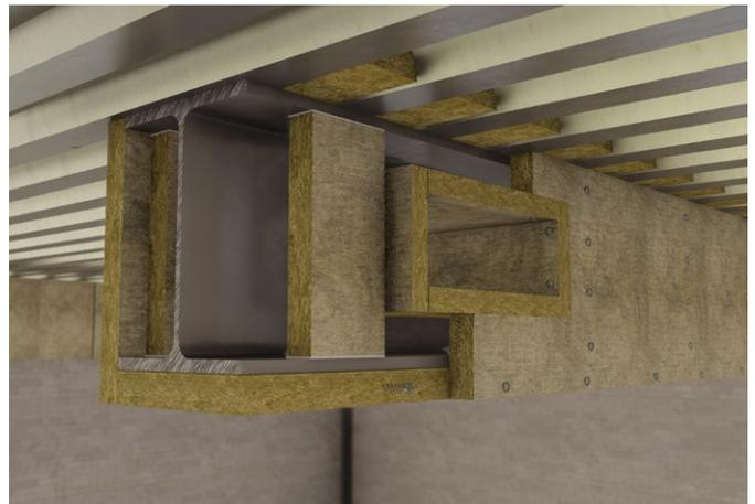
**Figure 14** - Beam with square or rectangular holes
