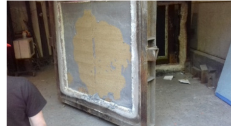
Back of test sample after two hours testing showing the furnace exposed face of the Fusion insulation
